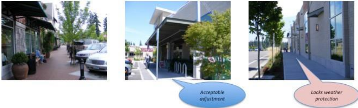
Left photo: Optimal compliance per subsection 5.13(2)(j). Right photo: Non-compliant; however, Middle photo shows potential Adjustments where additional weather protection is provided on side of building with greatest pedestrian use
