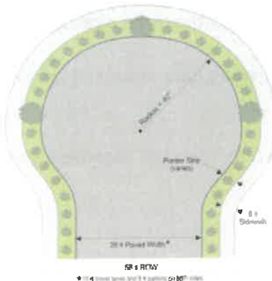
Figure 17. Cul-de-Sac Cross-Section Standards (this diagram applies to the local street cross-section)
