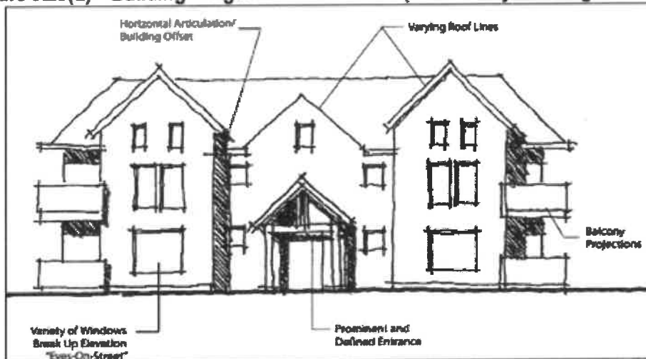
Figure 5.29(d) – Building Length and Articulation (Multi-family Housing Example)
